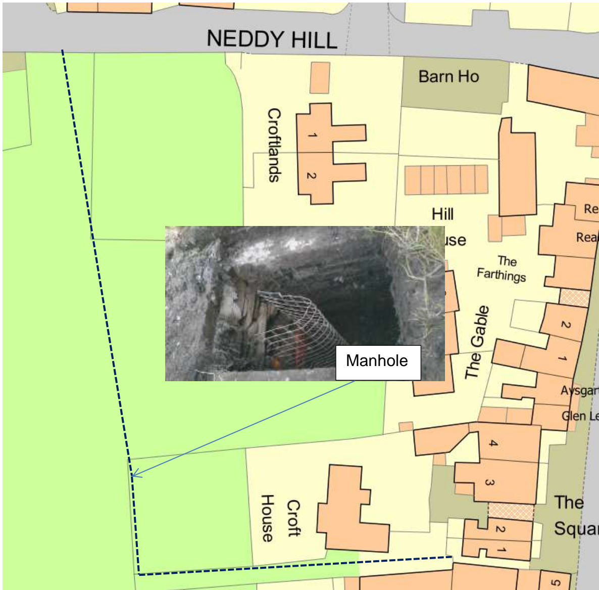
Figure 16: Charted route by highways in 2002 of drainage from The Square to NEDDY HILL.
